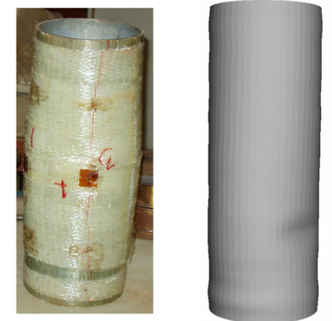
Fig. 16. Failure modes of FRP-confined steel tubes: finite element analysis versus experiment: (a) Tube ST-F1, (b) Tube ST-F2 and (c) Tube ST-F3.
