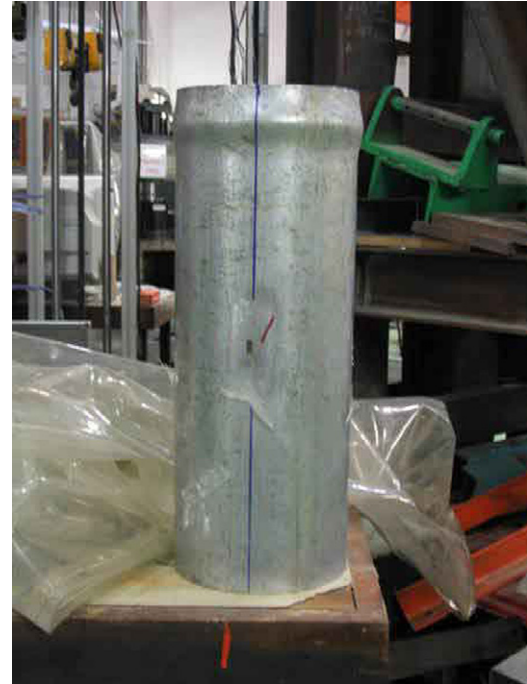
Fig. 4. Bare steel tube after compression test.
