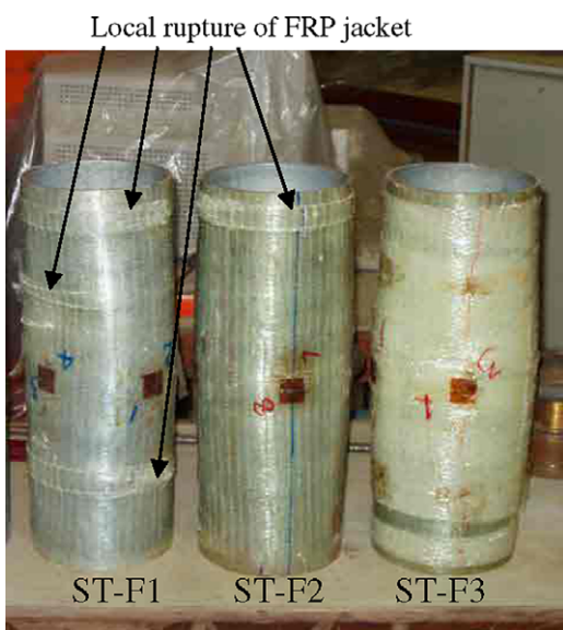
Fig. 6. FRP-confined steel tubes after compression test.
