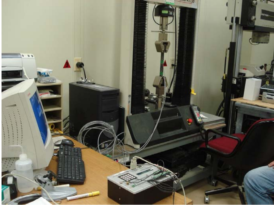
Figure 3 - Extension test of the composite laminate with strain gauges
