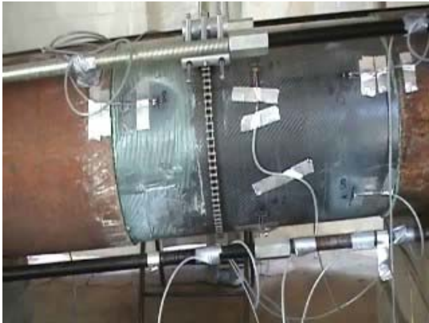
Figure 7 - The 16-inch pipe specimen during testing
