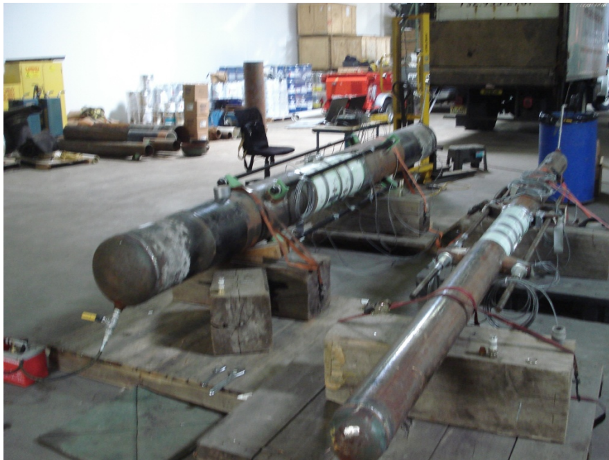
Figure 10 - The 12-inch and 6-inch pipe specimens
