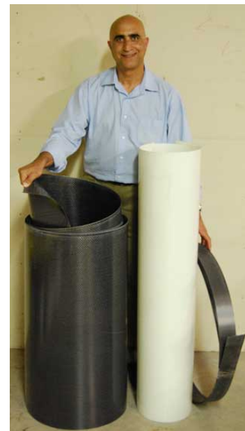
Fig. 2 - From left to right: Carbon and glass super laminates; carbon strip
